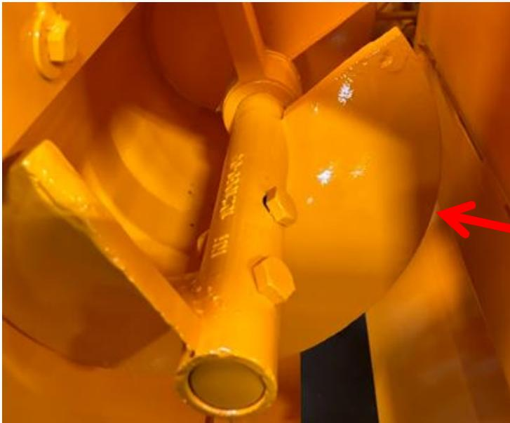
Temporarily remove the outer single auger from the assembly.
