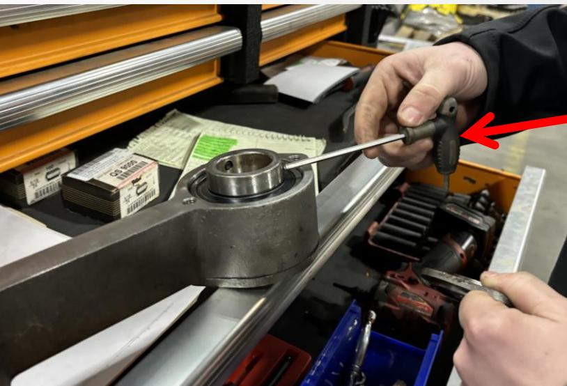
When the inside of the bearing is exposed, ensure that the shown set screws are still properly fastened. If the set screws are no longer in the bearings, then use the hardware that was provided to hold the auger in place.
