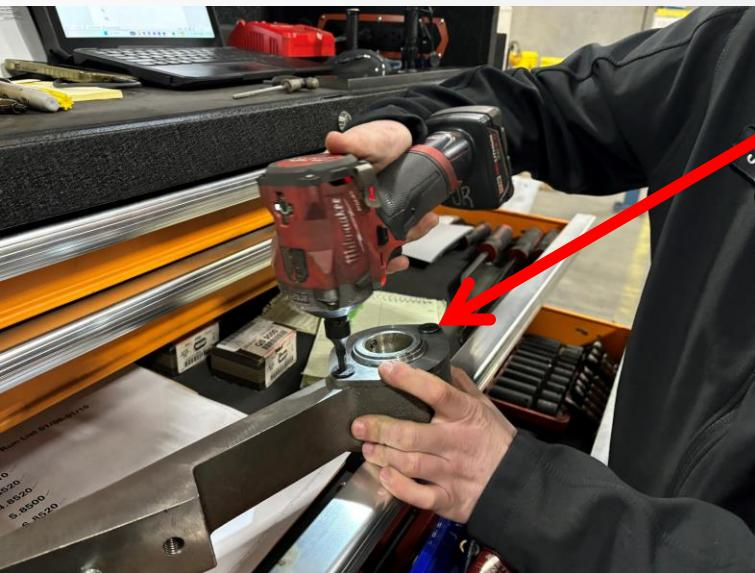
When the outer face of the bearing is exposed, unfasten the cover on the bearing.
