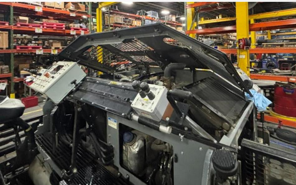
Continue firmly pressing the trim onto the outer perimeter of the hood assembly, until there is a 2" gap left on the other side.
