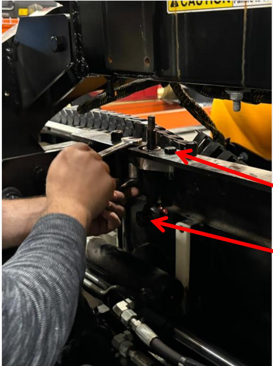
Paint the outer edges of the new bearing, before placing it onto the adjuster screw.
