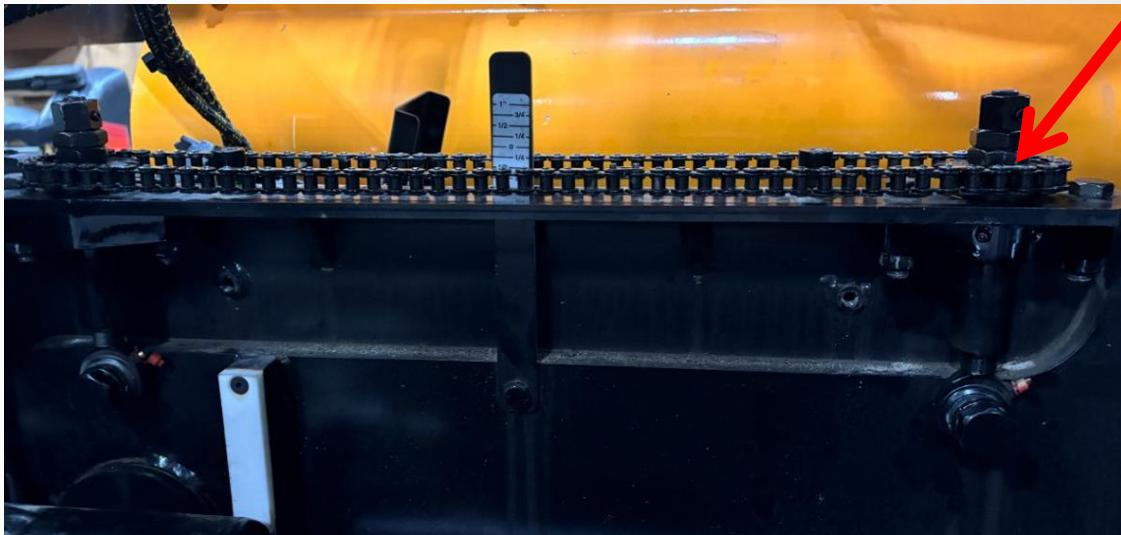
Fasten the new roller chain around the sprockets.
