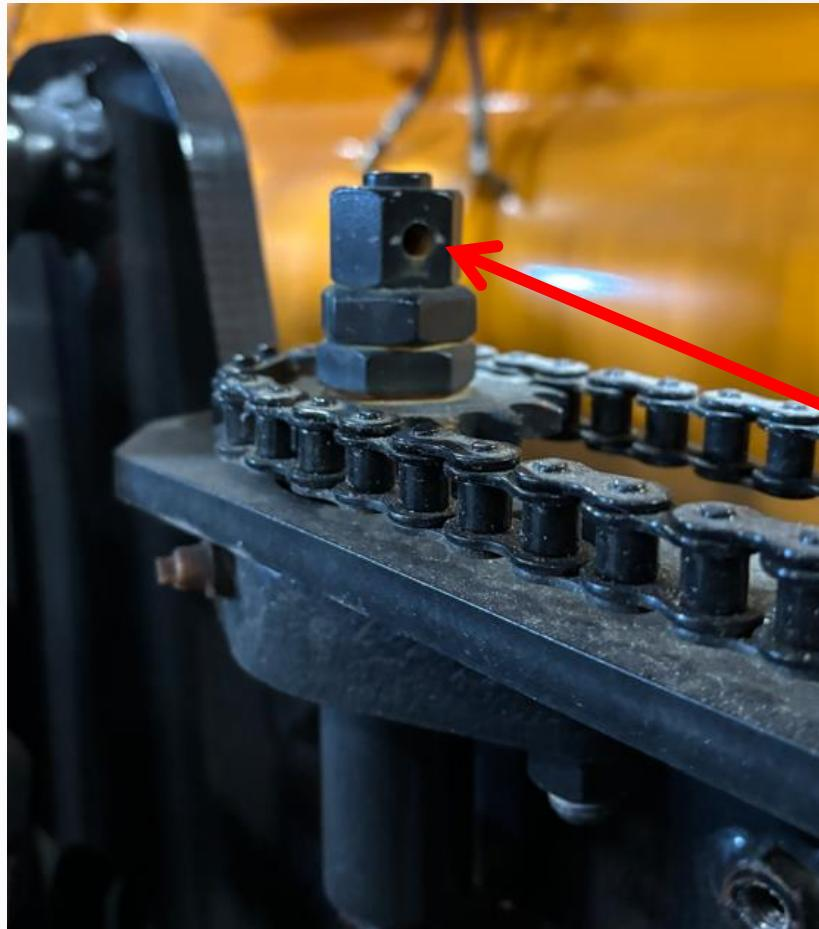
Temporarily remove the roll pin from the top of each vertical assembly adjuster.
