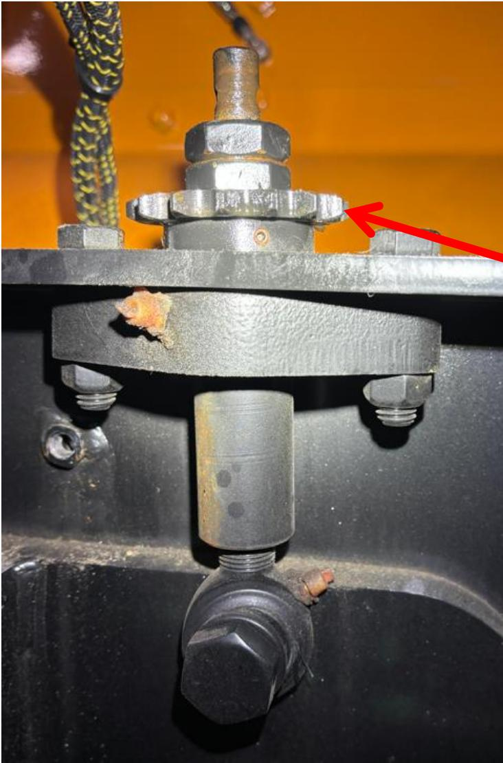
Refasten the sprocket and the two jam nuts back onto the top of the adjuster. Repeat the same process for the other bearing on the same side of the machine.
