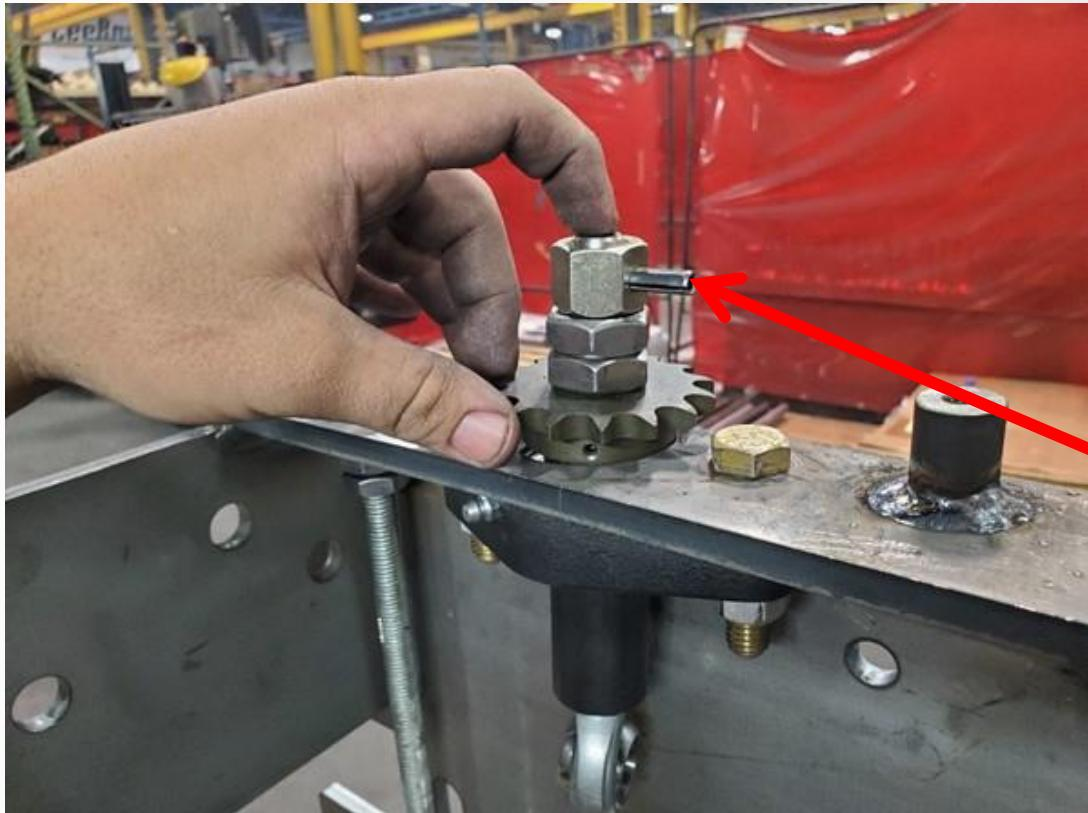
Place the set nut on top of the adjuster assembly and align the holes between the two components.
