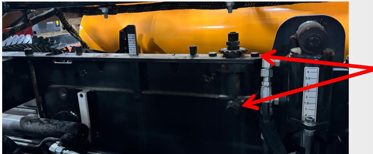
Next, loosen the hardware for one of the vertical screw adjusters, and remove the chain roller.
