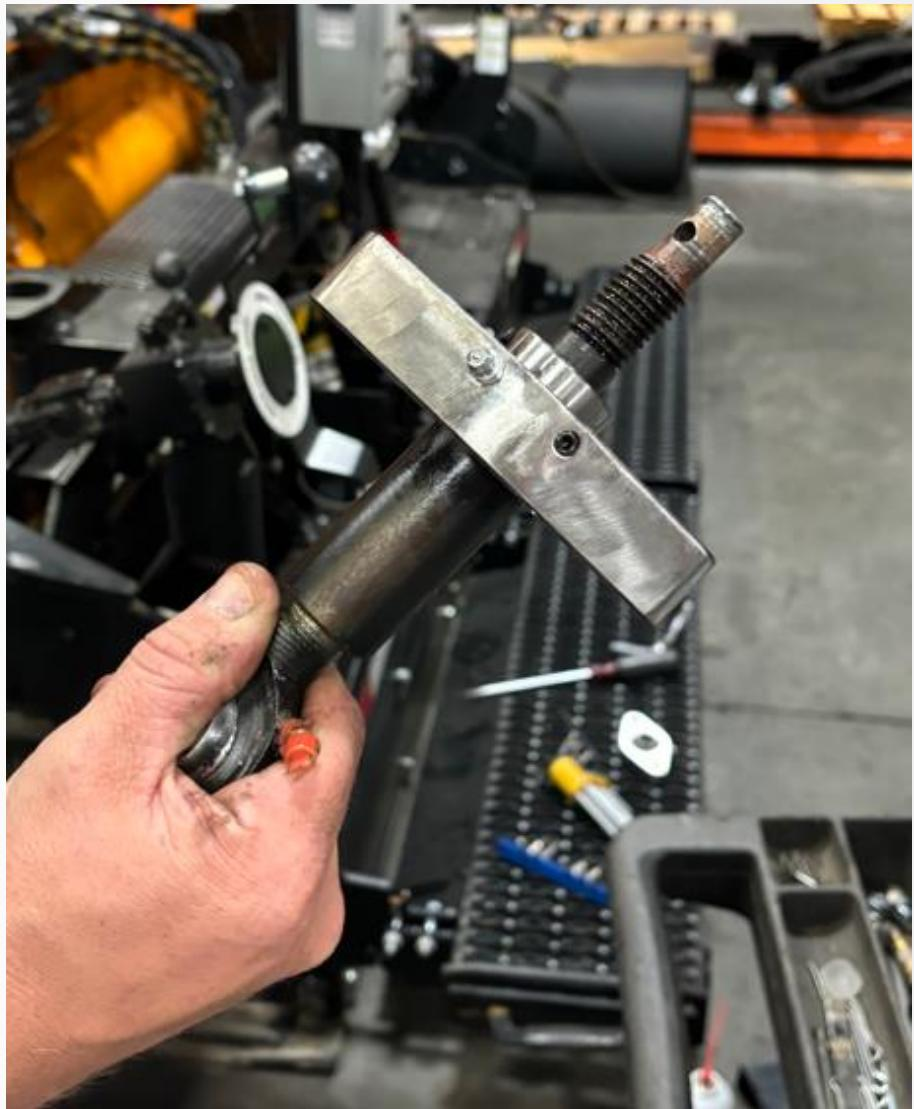
Unfasten the jam nuts, that are on top of the adjuster assembly.
