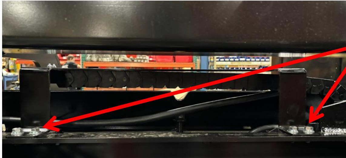
Remove the bolts that are holding the E-Chain support bracket.
