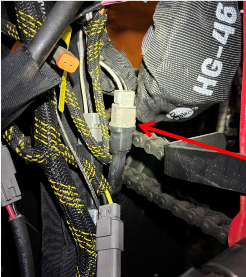
Use the provided contact cleaner to properly clean the existing electrical terminals, for the heating elements.
