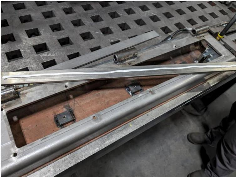
Locate the two tubes of the 2 oz. element transfer (PN# 986946). Carefully apply the paste to the bottom side of the S-Curve element.
