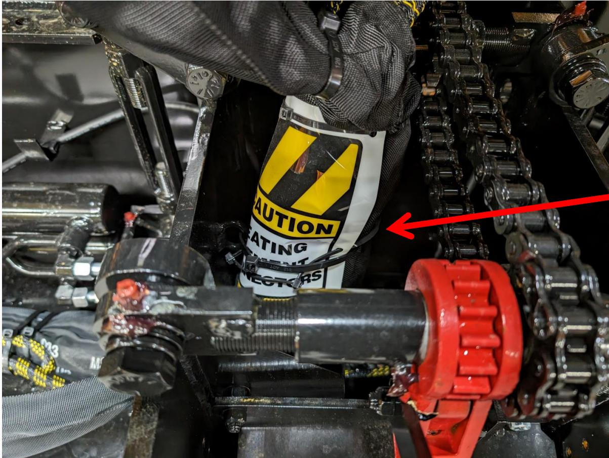
All element electrical connections can be found next to the crown and valley adjustments, in the center of the screed.
