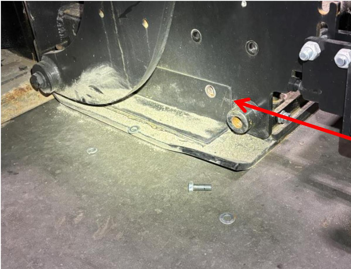
Next, remove the cover plate on the side of the main screed. This is where the S-Curve element will slide out.
