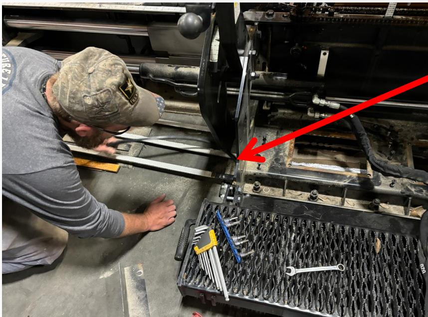
Insert the new s-curve element through the hole in the corresponding side of the screed frame.
