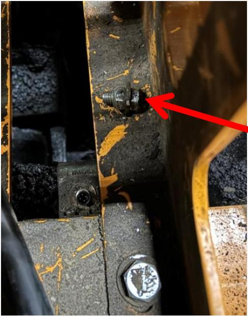
Remove the 3/8" hardware that is holding the paddle cable, to the toe board assembly.
