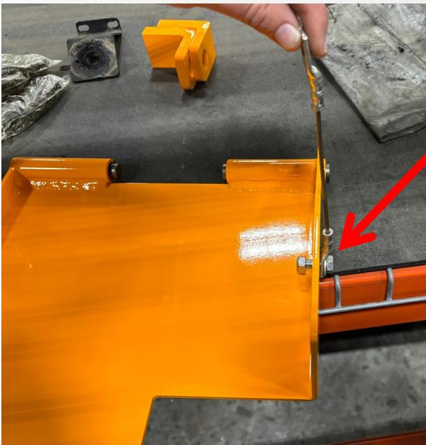
Use the new 3/8" hardware to loosely fasten one end of cable, to the side of the new paddle.
