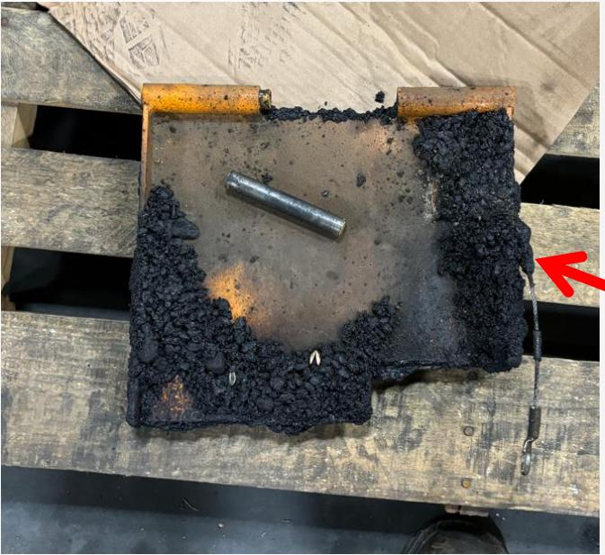
Pull the paddle, both pins and the cable, out of the paver assembly.
