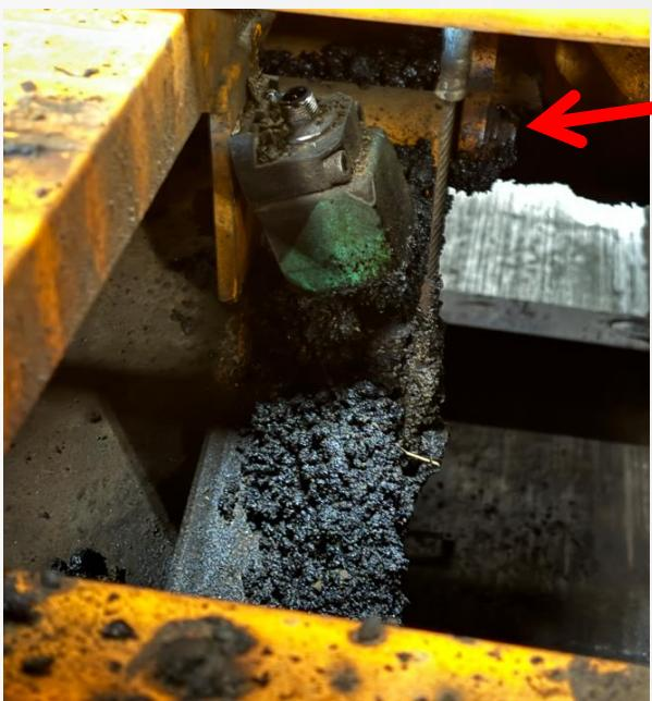
Unfasten the 7/16" hardware that is holding the paddle to the conveyor assembly.
