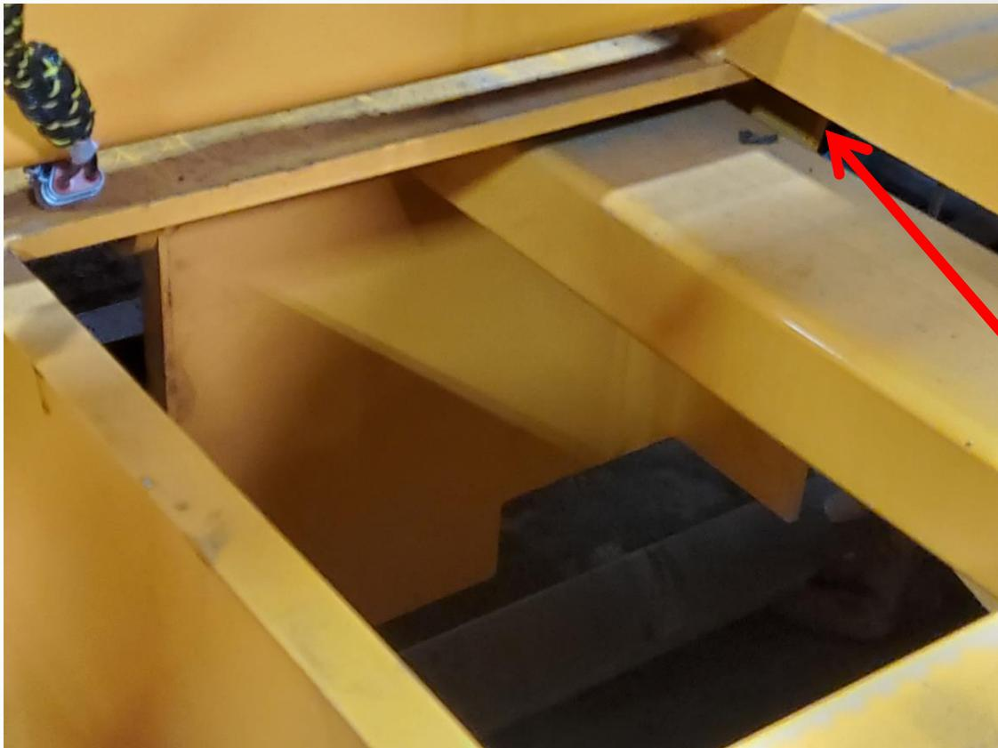
Insert the pins into the tube mounts, on the top side of the paddle.
