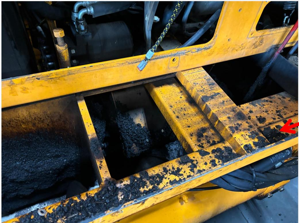
Remove the floor grating on the LH side of the paver assembly.
