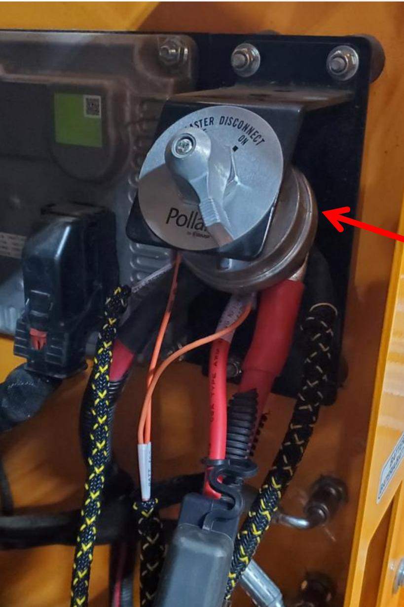
Open the RH Engine Cover Assembly, and locate the battery disconnect, that is attached to the top back.
