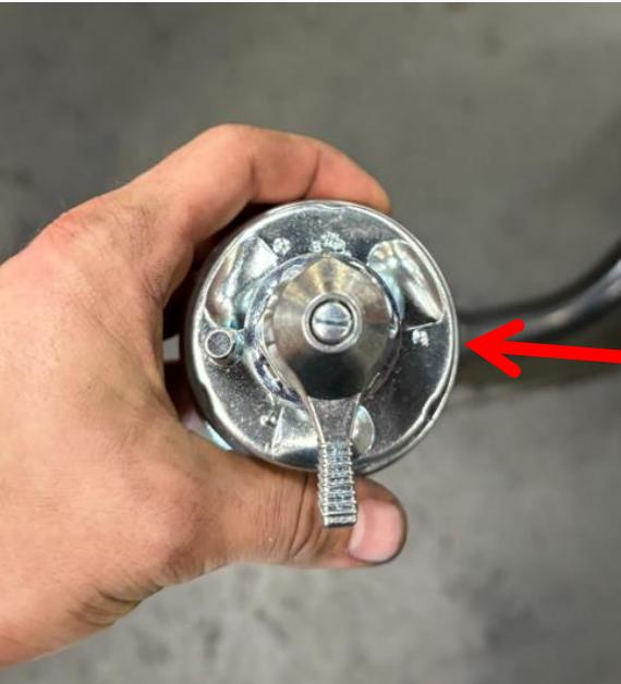
Remove every connection from the backside of the battery disconnect.
