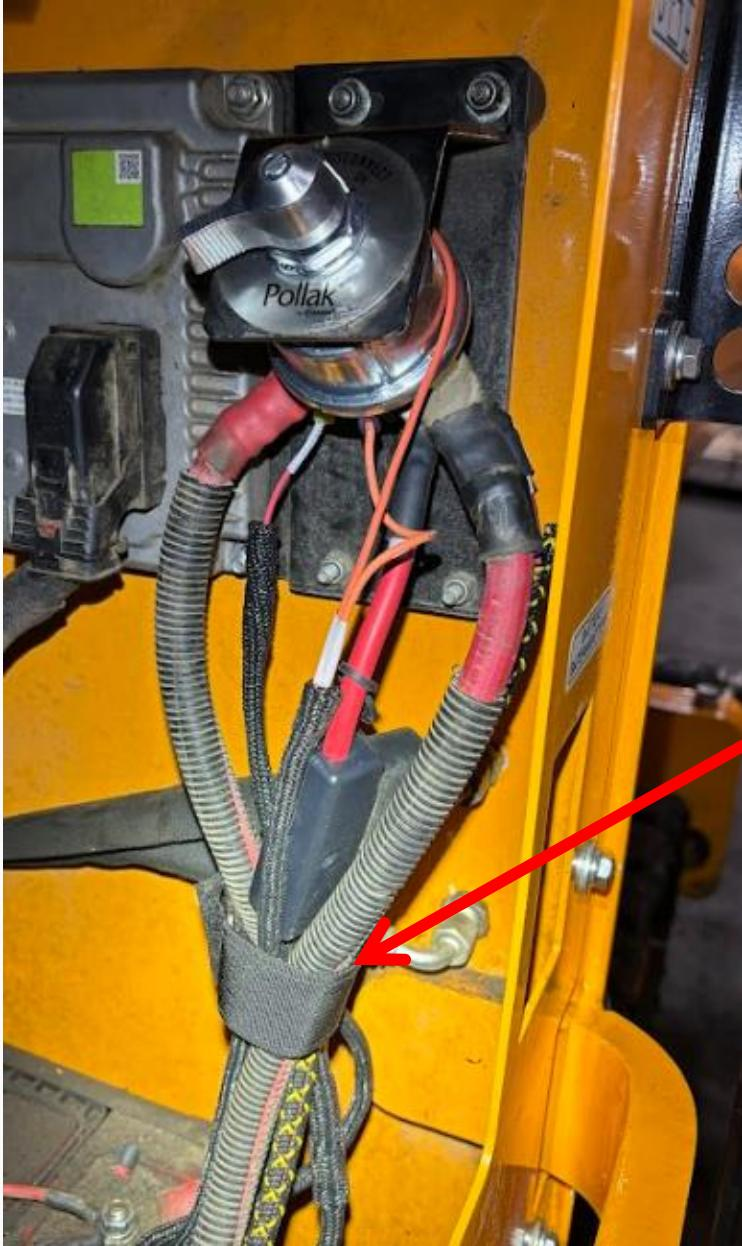
Use one of the 8" Velcro Cinch Straps, to securely hold the harness, below the battery disconnect.
