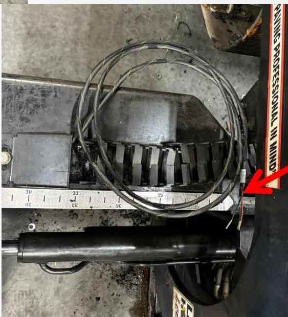
Route the loose end of the sonic wire through the e-chain, and through the ratcheting p-clamps along the bottom of the citrus tank.
