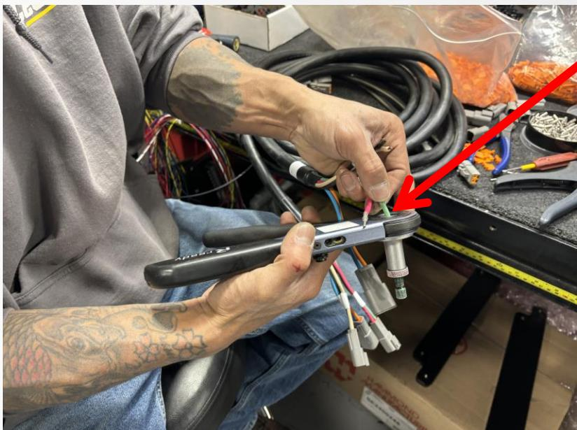
Properly crimp the 10-12AWG pin and socket terminals, to the ends of their designated wires.
