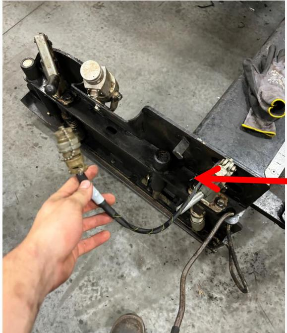
Locate the sonic sensor breakouts, included with the main screed harness.
