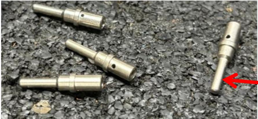
Locate the 10-12AWG pin and socket terminals that were supplied in the kit.
