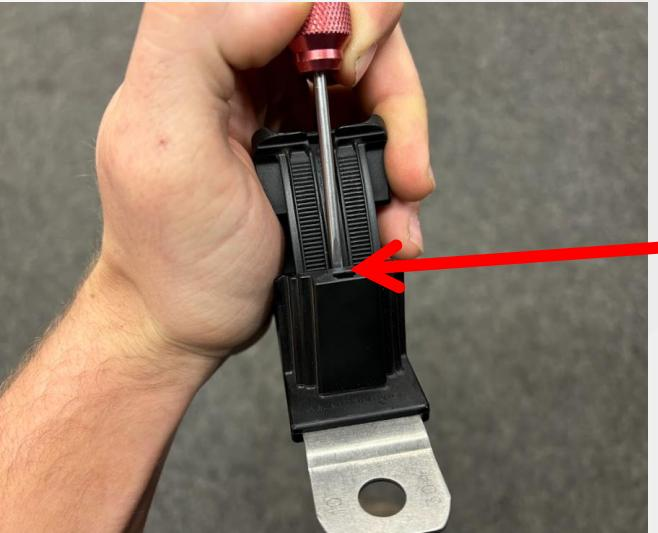
To successfully reopen the clamps, insert a zip tie or pin tool, in between the grooved strips and pull on the top jaw.
