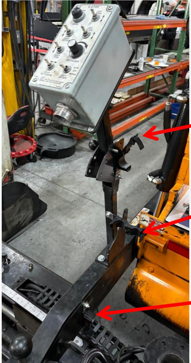
Locate the 1030263-C-180S-M10, ratcheting p-clamps, that came with the kit.
