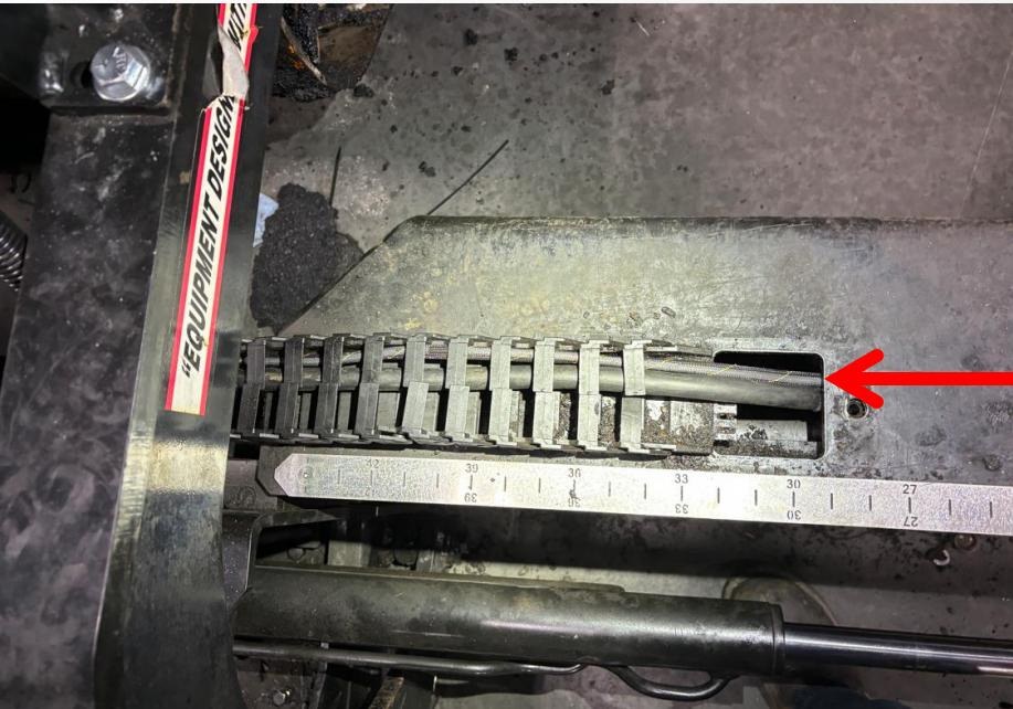
Insert the three terminals that are coming from the element harness, through the hole in the top of the extension.
