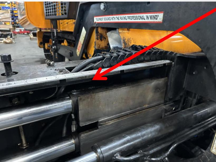
Insert the “ENG” breakout, on top of the wire cover, that is welded inside the extension.
