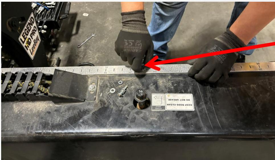
When the holes have been properly aligned, use the supplied hardware to securely fasten the rulers to the top side of each extension.
