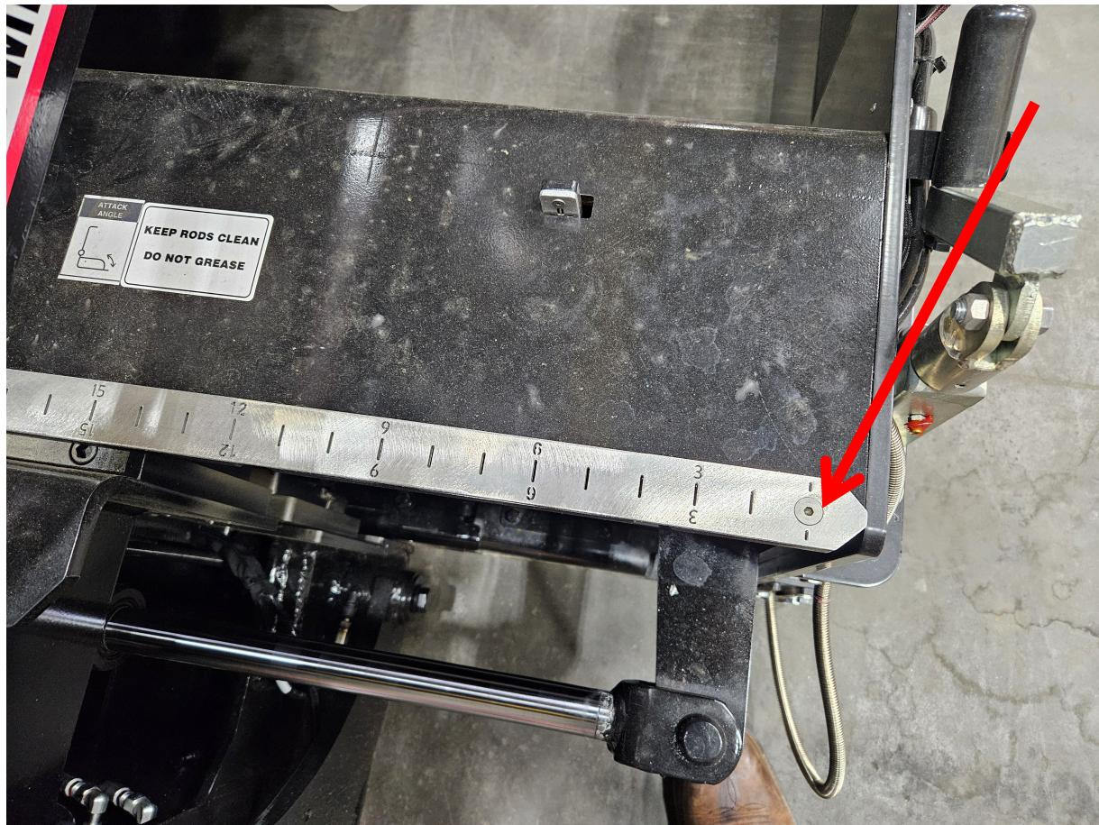
When the hardware has been securely fastened, ensure that the heads of the countersunk bolts are not sitting above the top of the extension ruler.
